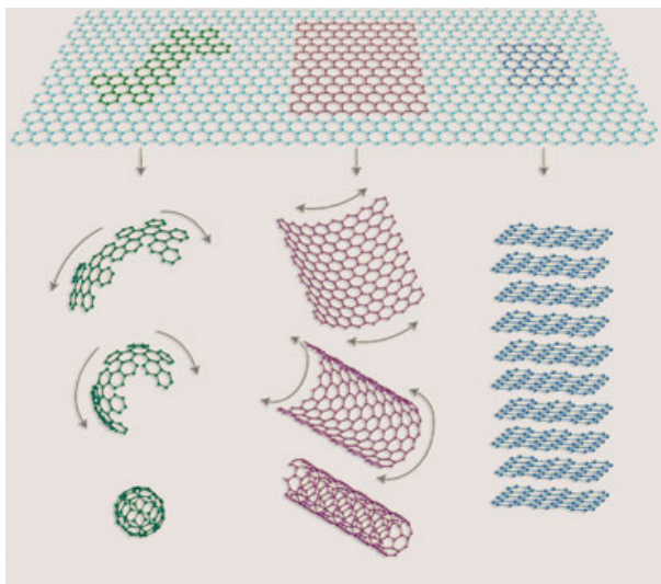
Graphene as a building block for carbon structures: (1) Bucky Balls (2) Nanotubes (3) Graphite
